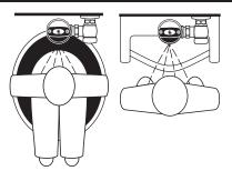
When the user steps away, the loss of reflected light initiates an electrical "one-time" signal that activates the flushing cycle to flush the fixture. The Circuit automatically resets and is ready for the next user.
