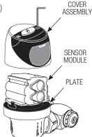
Install Battery Compartment Cover and secure with Retaining Screw.
