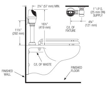
When installing the Optima Plus in a handicap stall:
